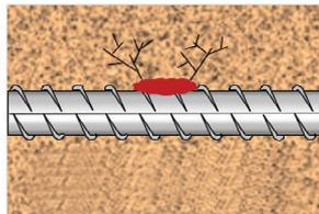
Stage 2: Crack propagation due to rust expansion
