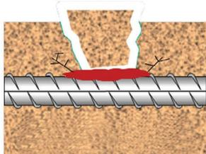
Stage 3: Concrete spalling after extensive cracking
